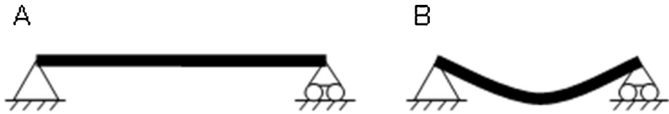
Fig. 7. (A) flat stationary plate, (B) bent plate due to vibration.
